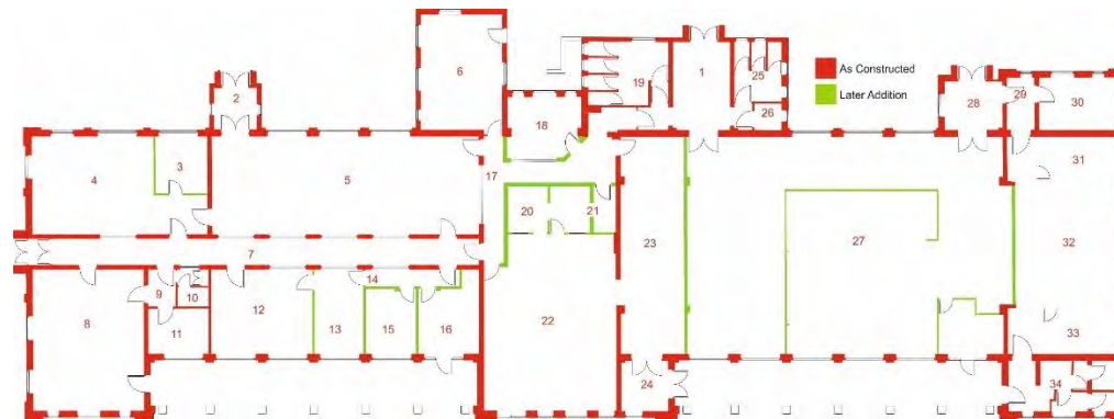
Figure 6 The layout of the Canteen Building
